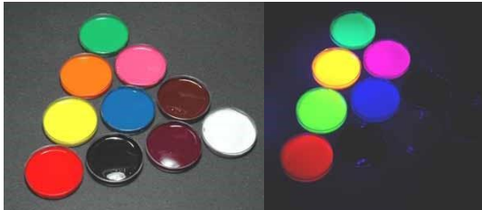
Figure 1: Samples of the ten VIE colors under ambient light (left) and illuminated by the VI light (right). Note that only the six fluorescent colors show up with the VI light, and that the colors, especially yellow, appear differently.
