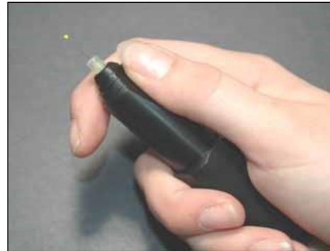
Figure 4: Manual Elastomer Injector, ready for tagging.
