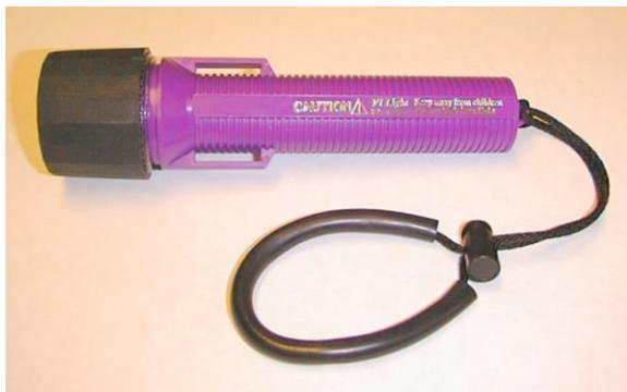
The VI Light (above) is used to fluoresce VIE and VI Alpha Tags. It has a nearly invisible, regulated, deep-violet beam. Deep violet (405 nm) is the optimum wavelength for fluorescing our tags.
